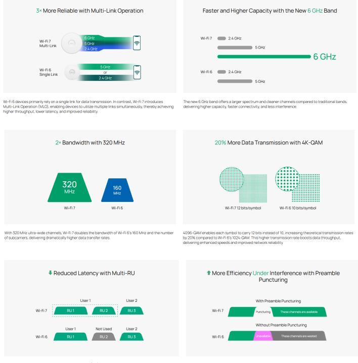
Wi-Fi 6 restricts each user to a single resource unit (RU), limiting spectrum flexibility. Wi-Fi 7 overcomes this limitation by allowing multiple RUs to be allocated to a single user and enabling RU aggregation, improving data throughput and spectral efficiency. Preamble puncturing identifies and excludes interference-affected subcarriers, reducing spectral waste and boosting efficiency in challenging wireless conditions.
